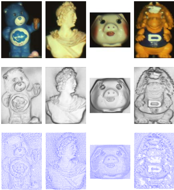
Figure 3. First row: Polarised images of sample real-world objects; Middle row: Recovered shading maps; Bottom row: Needle maps yielded by our method.
