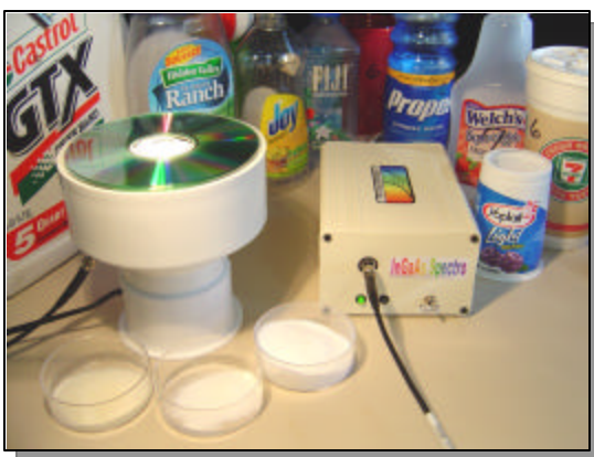
Fig.2: StellarNet EPP2000-NIR-InGaAs spectrometer used to capture sample reflectance spectra shown in the graphs.
